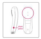
4. Short press the power button/mode button on the side of the device to turn it on. The default mode is Fast Mode, and the cooling function will be active during the whole process, so the relevant indicators will be on when the device is turned on.
