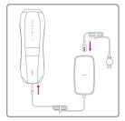
1. Connect the power cord, power adapter and device as shown in figure.
