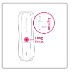
The device features two operating modes: auto mode and manual mode. In automatic mode, the device automatically emits light pulses at regular intervals without requiring manual operation. In manual mode, the user must manually press the flash button to emit a light pulse. It's important to note that the SHR mode does not include an auto mode.
