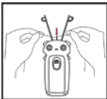
Step 1: Pass 36cm of cotton thread through the middle hole, keep the wire the same length on both sides.
