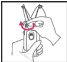
Step 4: Tighten the right thread then entwine in the bottom of the right knob, fasten the bolt.
